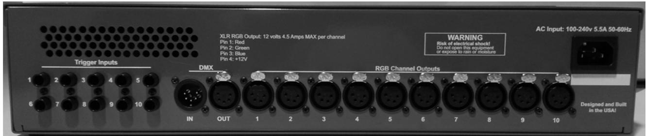
The back panel of the unit has 10 4-pin female XLR output connectors. Each connector will drive up to 4.5 amps at 12 volts for your LED's. The maximum draw from all channels at the same time must not exceed 29 amps.
