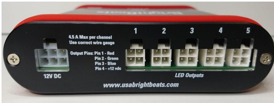
**If you are making your own cables be sure to use the proper gauge to minimize voltage drop and have the ampacity to safely carry the current for your LED's!**
