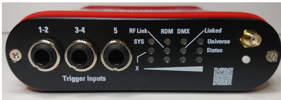
In general, the safe input range is from 0-12 volts. These inputs can be connected to various devices depending on how you wish to trigger the LED's. In addition to triggers, musical instruments, audio outs and similar devices can be used to trigger **but care must be taken not to overdrive the input or damage may occur.**
